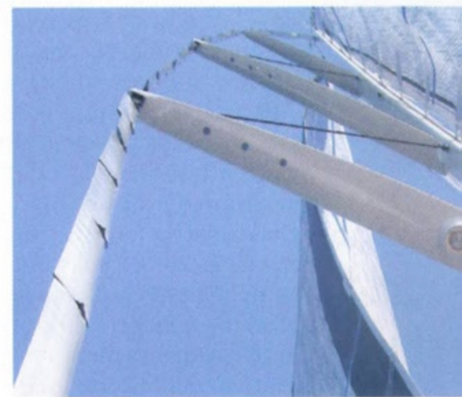
NACA sectioned fairings are each 2m long and free to rotate to the breeze. Note the different angles of attack up the rig
